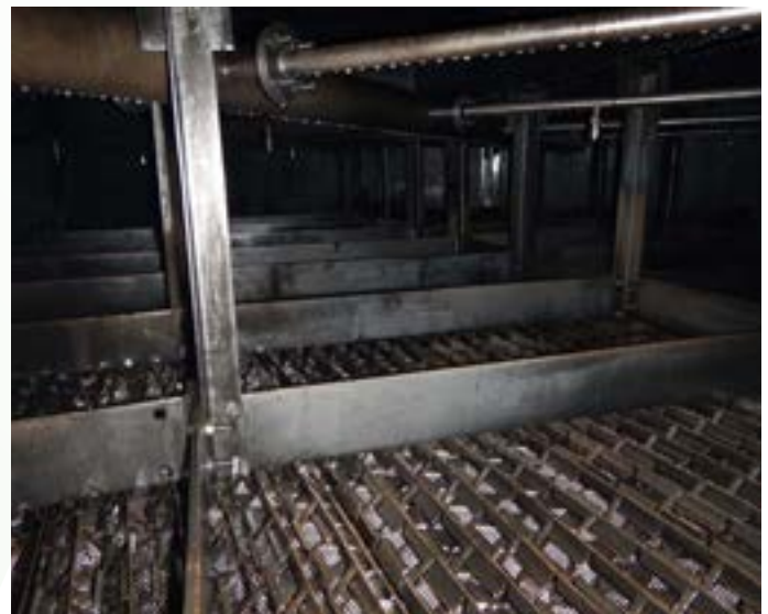
◆ VDU PACKED BED SECTIONS CONTAINED NO SCALE OR PYROPHORICS AFTER ZYMEFLOW'S PROCESS
